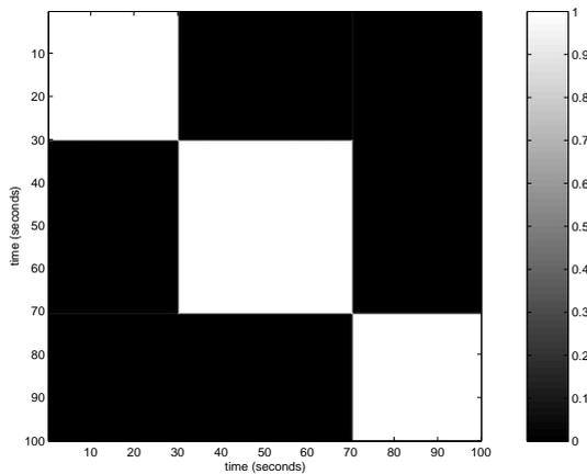
Figure 3: Similarity matrix for synthetic signal of Figure 2.
